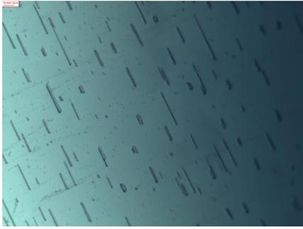
(a) Hydrogen annealing during the heating step, 20 sccm H<sub>2</sub> and 180 sccm Ar at 800 mTorr while heating to 800 °C in 30 minutes.
