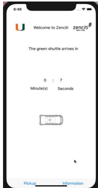
Figure 32: A timer which represents the waiting time until a shuttle arrives. If a user presses the button ,Information', a timer appears which indicates how long the passenger must wait for the arrival of the called shuttle.
