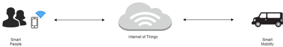
Figure 9: Smart Mobility simulation block diagram. People can easily communicate each shuttle, which is currently driving on the road via the Internet of Things. Data from the smartphone is collected via the installed smartphone application which is connected to the Internet as well.
