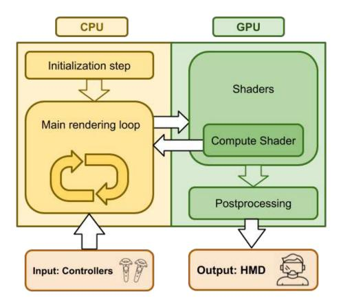
Figure 4.3: System Architecture Diagram
