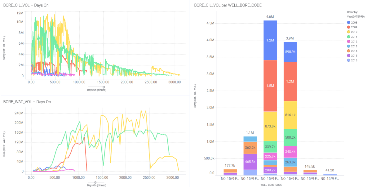
Figure 21: Oil and water production data from the Norwegian Volve field, per well and year (right) and normalized to days on stream (left), data from https://data.equinor.com/volve . Decline curve analysis implemented with R code (not shown).
