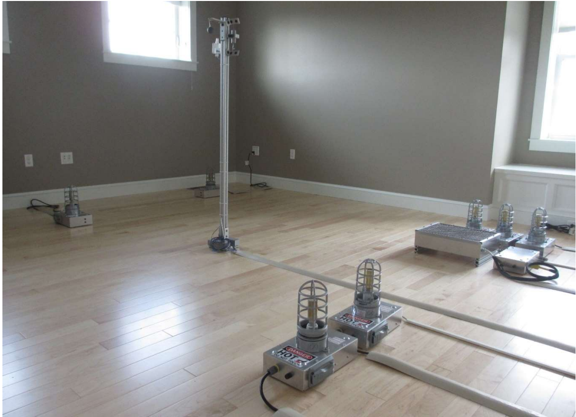
Figure 27: Resistance heaters, sensors for dry air temp, relative humidity and radiant temperature (NIST)
