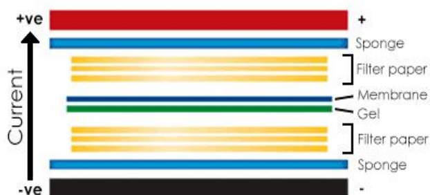
Figure 3, Western blot stack for transferring proteins onto the membrane. (abcam.com/protocols/general-western-blot-protocol, Access date: 5.20.2019)
