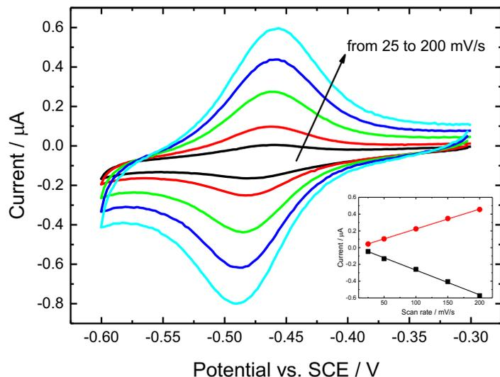
Figure 1. Typical cyclic voltammograms at AQ-modified gold electrode in 0.1 M phosphate buffer (pH 7). The electrode potential was swept from -0.3 to -0.6 V vs. SCE (5 cycles) at different scan rates: 25, 50, 100, 150 and 200 mV/s. The inset shows a plot of the peak currents as a function of scan rate. This plot was used as a reference to test the amino-modification using anthraquinone-2-carboxylic acid solution.
