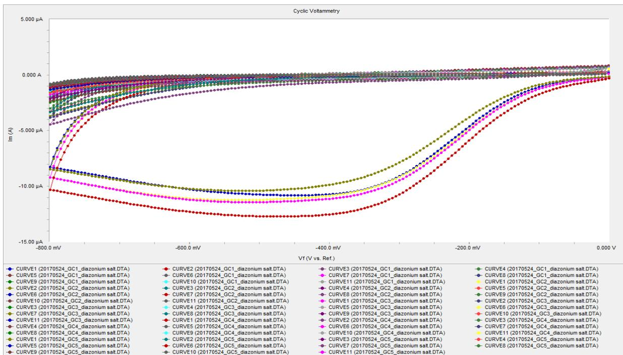
Figure 4. Example of the diazonium salt reduction on the electrode. These data were also from the last experiment described in session 3.5, but they clearly showed the reaction process.
