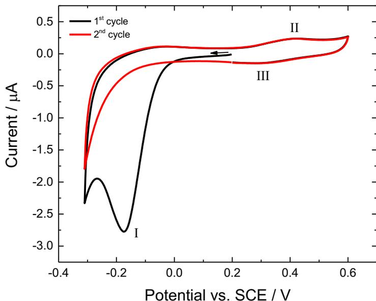
Figure 2. Typical cyclic voltammograms at NTP-modified gold electrode in 0.5 M sulfuric acid. The electrode potential was swept from 0.2 to -0.3 V, and then to 0.6 vs. SCE at 50 mV/s. This plot was used as a reference to test the maleimide modification using nitrothiophenol.
