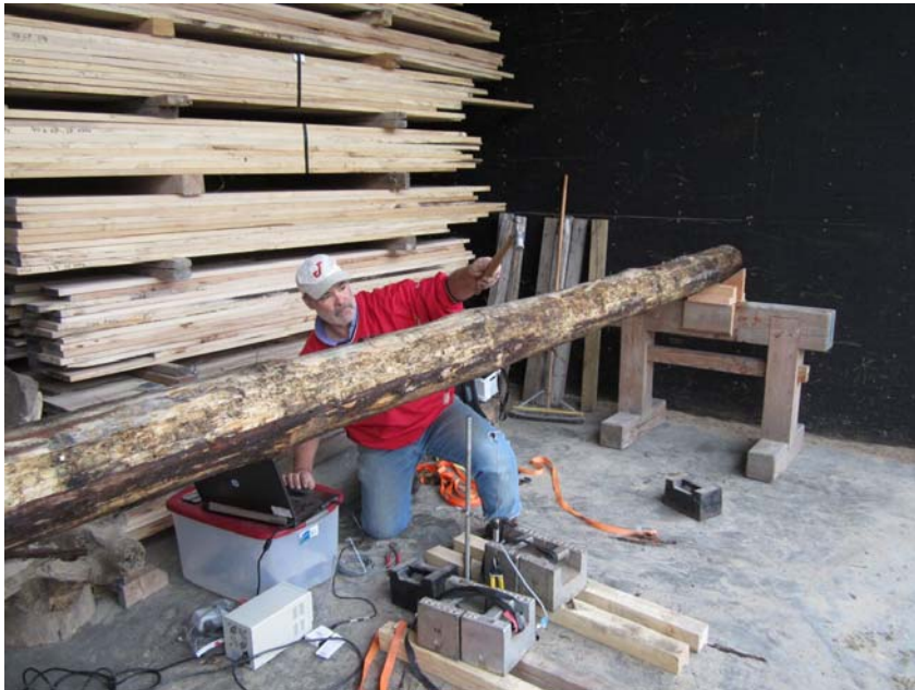
Figure 3 Experimental setup for transverse vibration measurement
