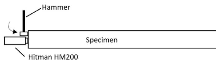
Figure 2 Experimental setup for stress-wave measurement
