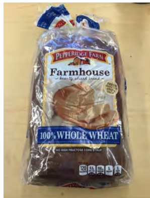
Fig. 6. Loaf of bread that is completely packaged; wrapped in an inner layer of BOPP and placed into an outer bag of LDPE
