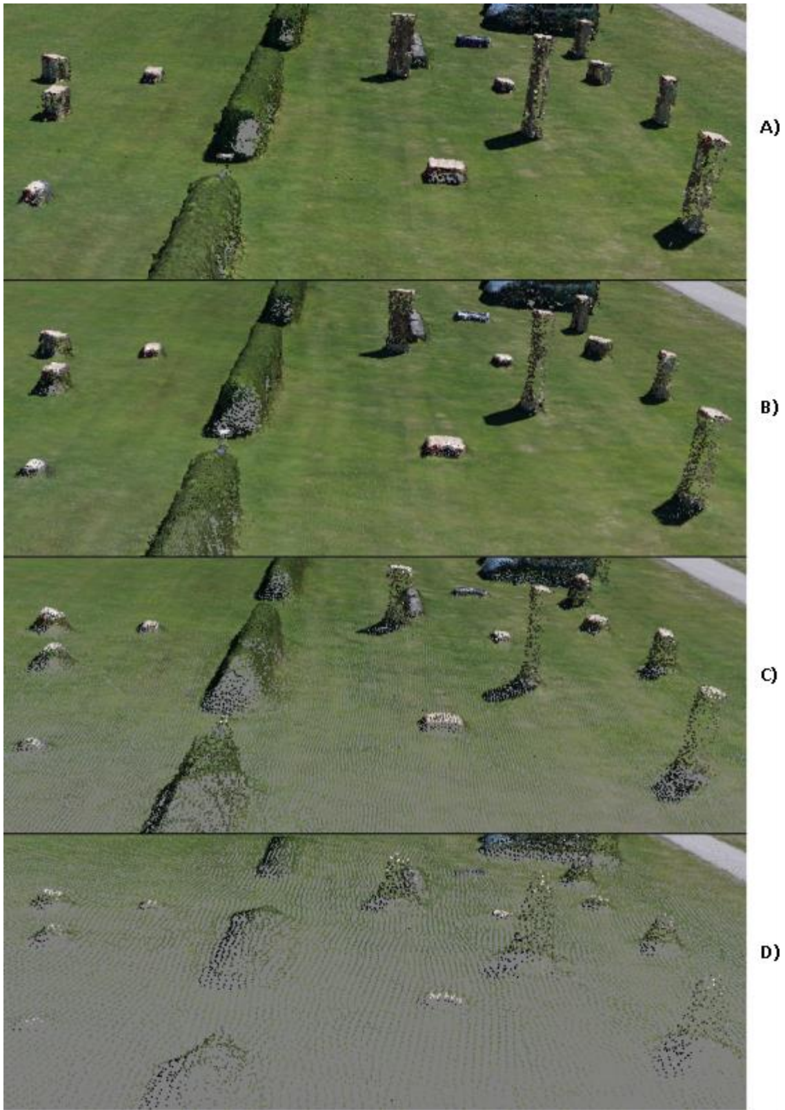
Figure 9:: Examples of the four different point cloud densities from Flight 2. A) Ultra-high density, B) High density, C) Medium density, D) Low density
