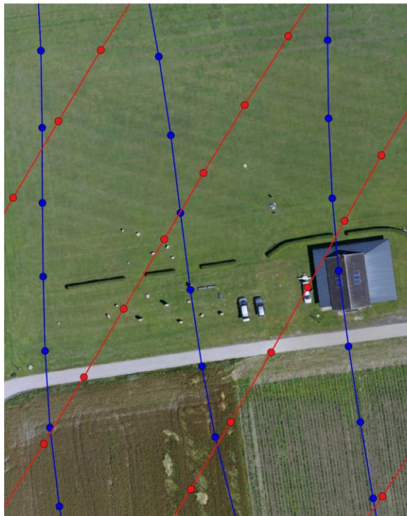
Figure 7: The four flight paths and camera locations, as flown. A) Shows the adapted RSI method, B) shows flight path shifted by 30 degrees compared to original, C) shows flight path shifted 60 degrees compared to original.
