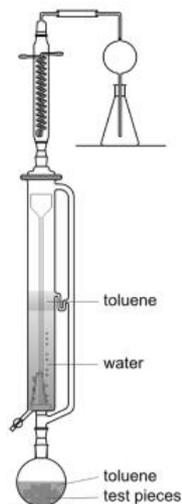
Figure 2: Perforator apparatus, Source: <https://www.scienceopen.com>
