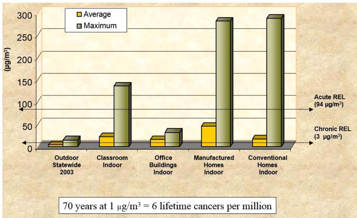
Figure 1: Typical formaldehyde levels, Source: Proposed Airborne Toxic Control Measure 26.4.2007
