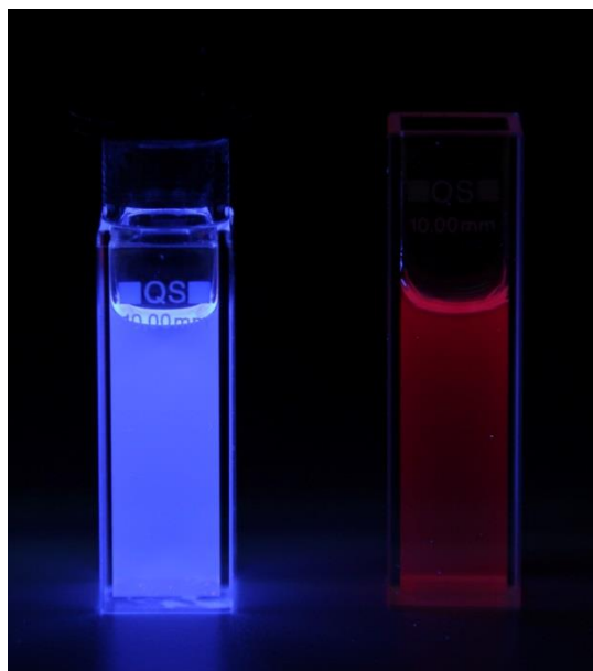
Figure 5.5 Dissolved conjugated polymers (left) and conjugated polymer-based nanoparticles (right) under UV light.
