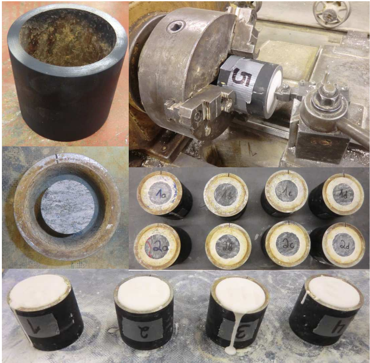
Figure 16: Casting and grinding of the PPT samples
