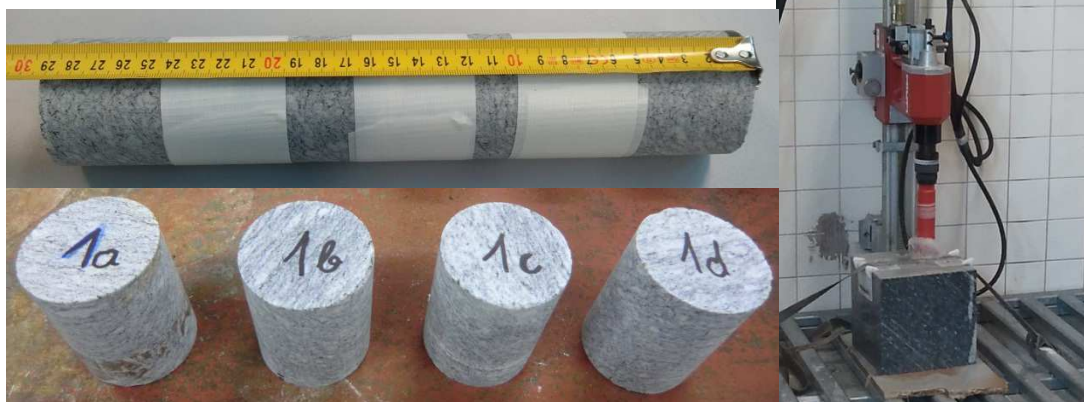
Figure 15: Preparation of rock cores
