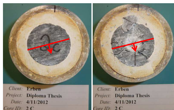
Figure 34: Failure along schistosity planes (Augen Gneiss)
