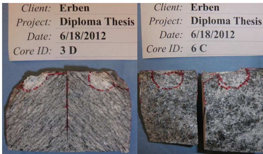
Figure 48: Growth of the SCZ with depth: Augen Gneiss (3); Calcareous Mica Schist (6)
