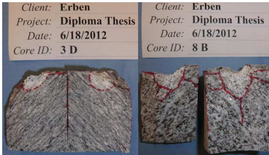
Figure 50: Propagation of the SCZ in direction of foliation: Augen Gneiss (3); Granite Gneiss (8)
