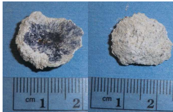
Figure 38: Primary crushed zone (Imberg)
