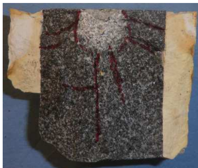
Figure 51: Crack pattern after a PPT
