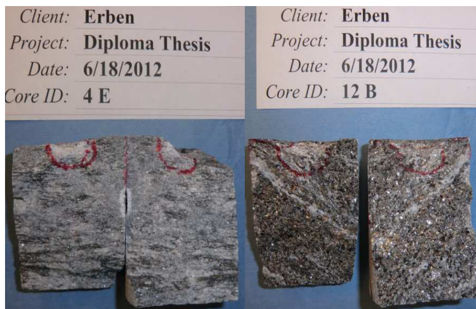
Figure 49: Shallower secondary crushed zone in ductile rocks: Calcareous Mica Schist (4); Schist Gneiss (12)
