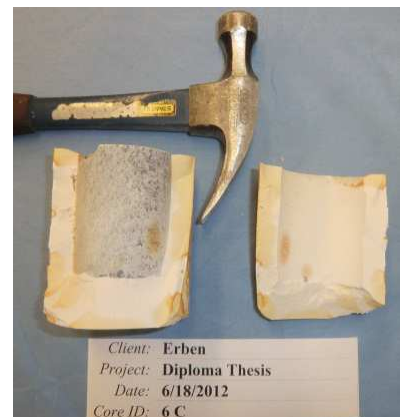
Figure 39: Breaking the Hydrostone with a geologist's hammer
