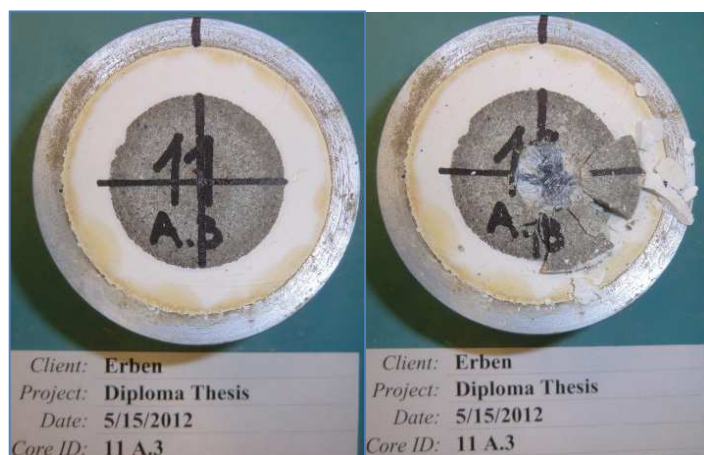
Figure 33: Indenter pressure enlarges the line width (Imberg Sandstone)
