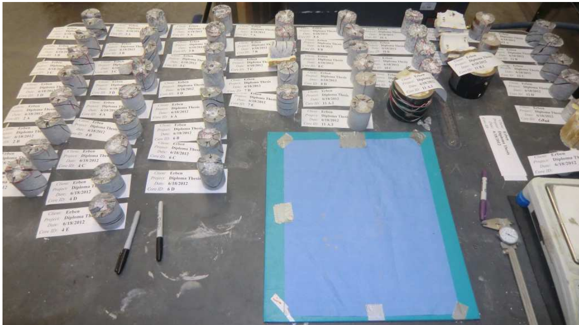
Figure 52: "Unwrapped", marked and split samples
