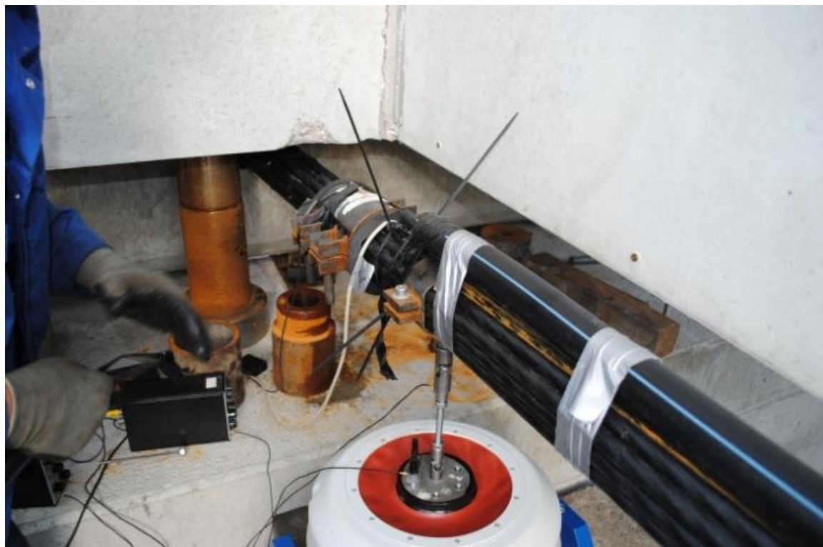
Figure 11. Damper and shaker connected to the stay cable
