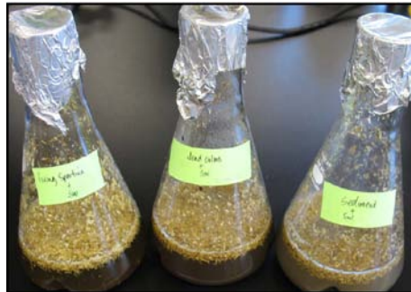
Figure 6 mesocosms to enrich the degradation community
