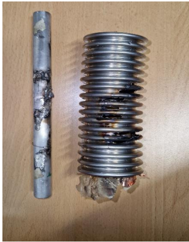
Conductor and cryostat for 5 kA LN2 measurement
