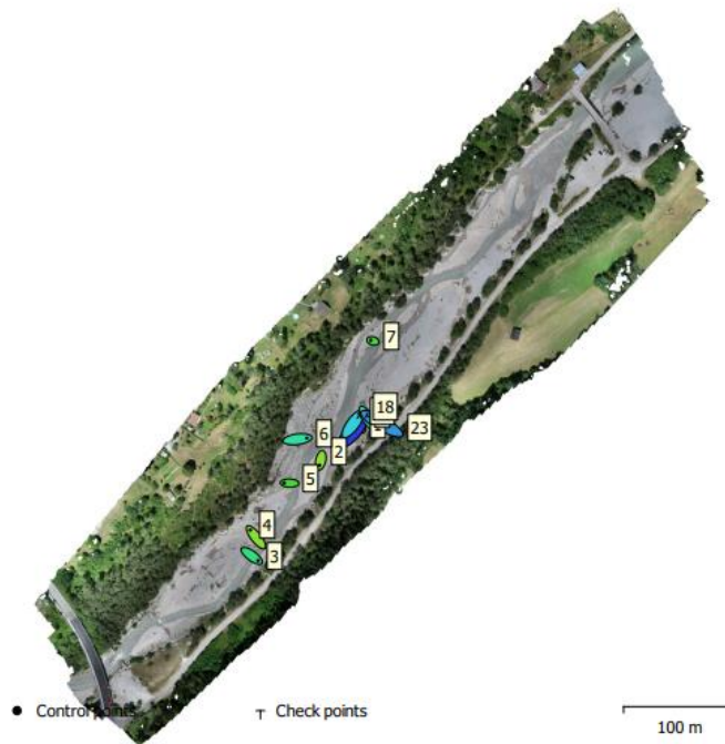
Figure 8 – The SfM orthoimage with control points and check points shown.
