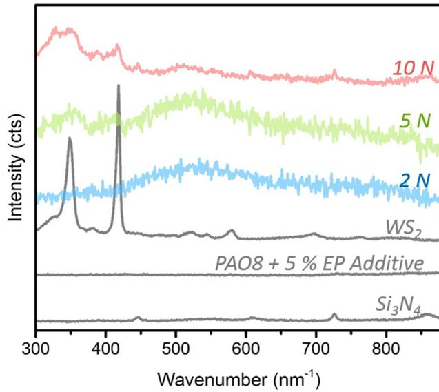
Figure 14: The WS<sub>2</sub> containing Tribofilms worn away under higher loads, leading to the continuous reproduction of bigger amounts of WS<sub>2</sub> debris and therefore easier detection by Raman spectroscopy.
