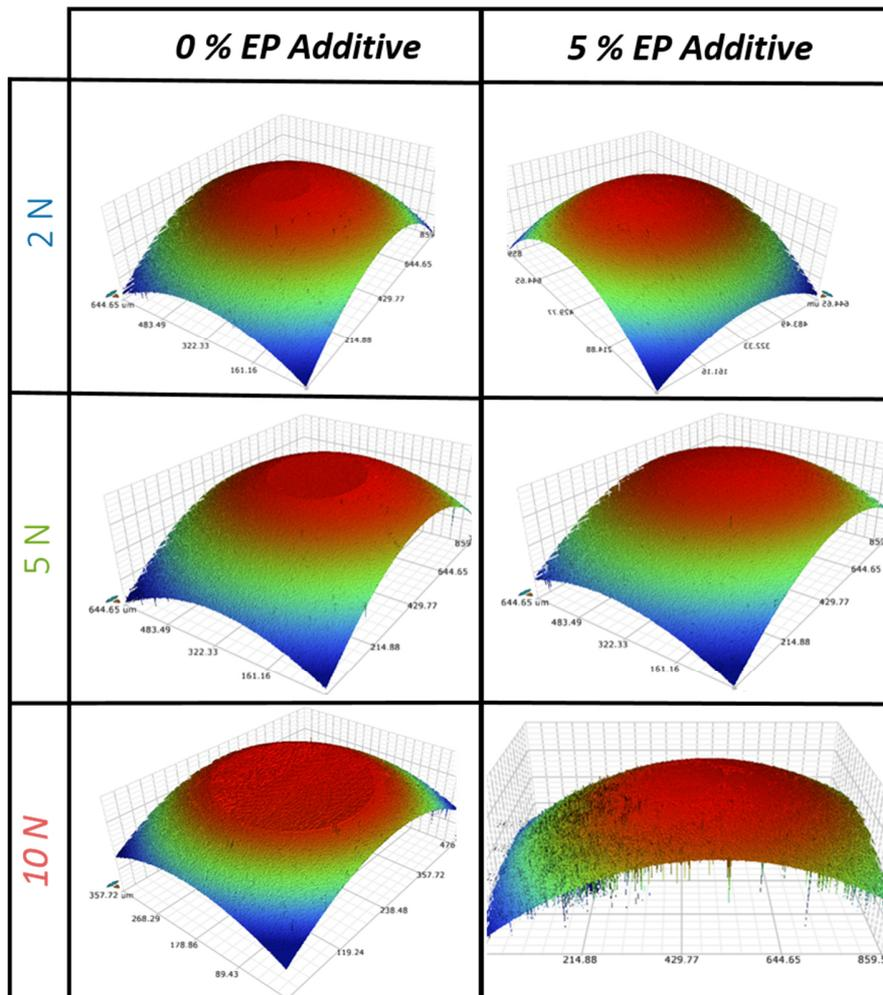
Figure 16: Even under higher loads that wear away the tribofilm the wear protection of the in-situ formation of  $WS_2$  still is operational.
