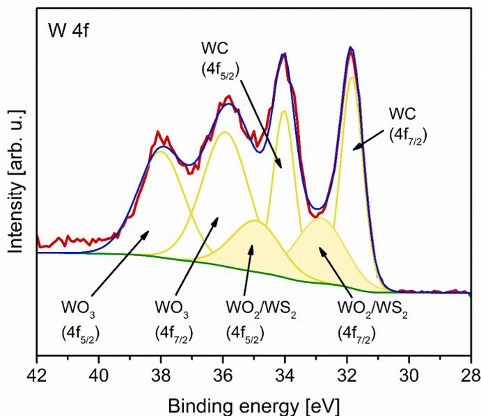
Figure 3: The W4f XPS scan of a tribocontact after the in-situ generation of WS<sub>2</sub>, demonstrating the difficulty of overlapping signals with WO<sub>2</sub>.
