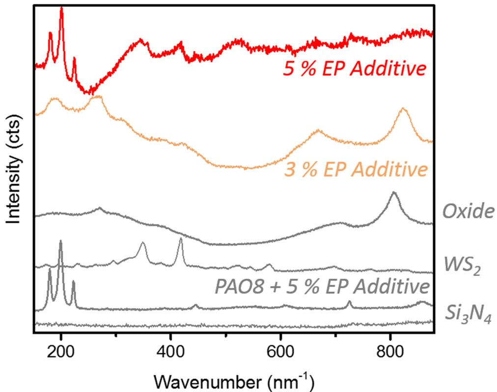
Figure 10: Due to the availability of oxides a WS<sub>2</sub> based tribofilm can form, as shown by Raman spectroscopy and lubricate the contact.
