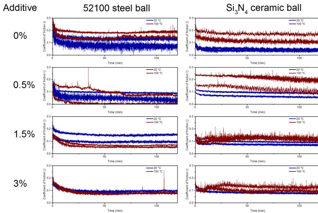
Figure 4: The coefficient of friction of a  $\text{Si}_3\text{N}_4$ - and steel ball, respectively vs. a tungsten carbide flat demonstrating very unstable tribological behavior. The temperature plays a clear role in the behavior of the coefficient of friction.
