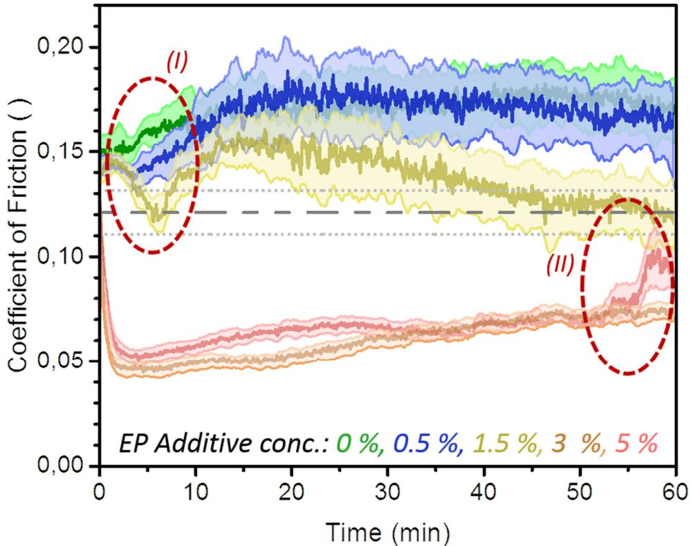
Figure 9: At high enough EP-additive concentrations a tribochemical reaction is induced, leading to a low friction regime which is clearly dependent on the availability of oxides.
