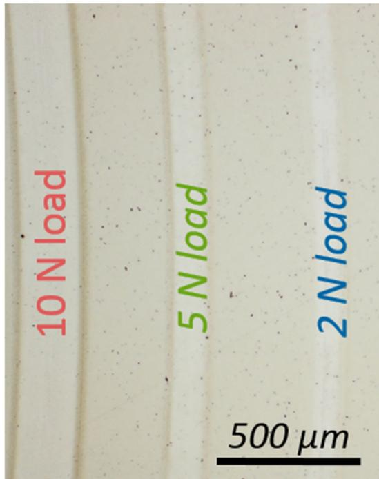
Figure 13: Debris is deposited on the sides of the wear track that does not show any significant wear.
