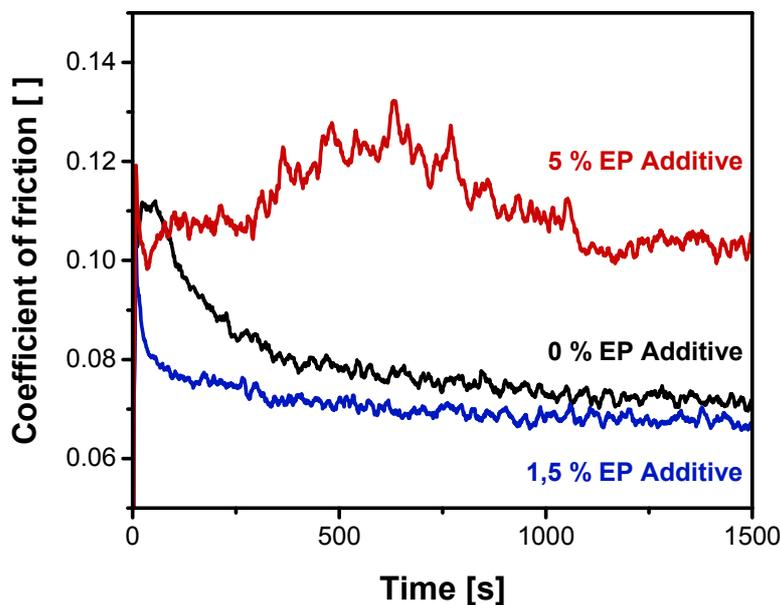
Figure 1: Evolution of the COF of a lubricated tungsten carbide coating against 100Cr6 steel ball contact at 10 N and the influence of the lubricants EP additive level.
