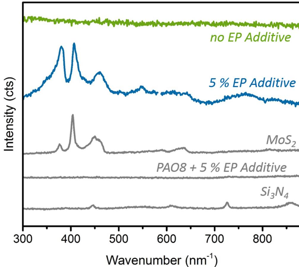
Figure 6: Raman spectra of the wear scars on Mo flats indicate that the EP additive leads to low friction due to the in-situ formation of MoS<sub>2</sub> in the contact.
