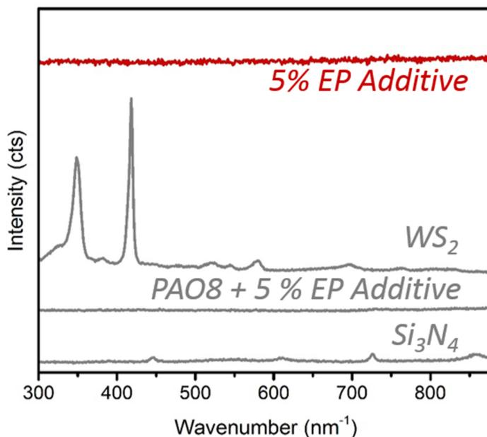
Figure 8: Raman spectroscopy supports the absence of in-situ formed  $WS_2$ .
