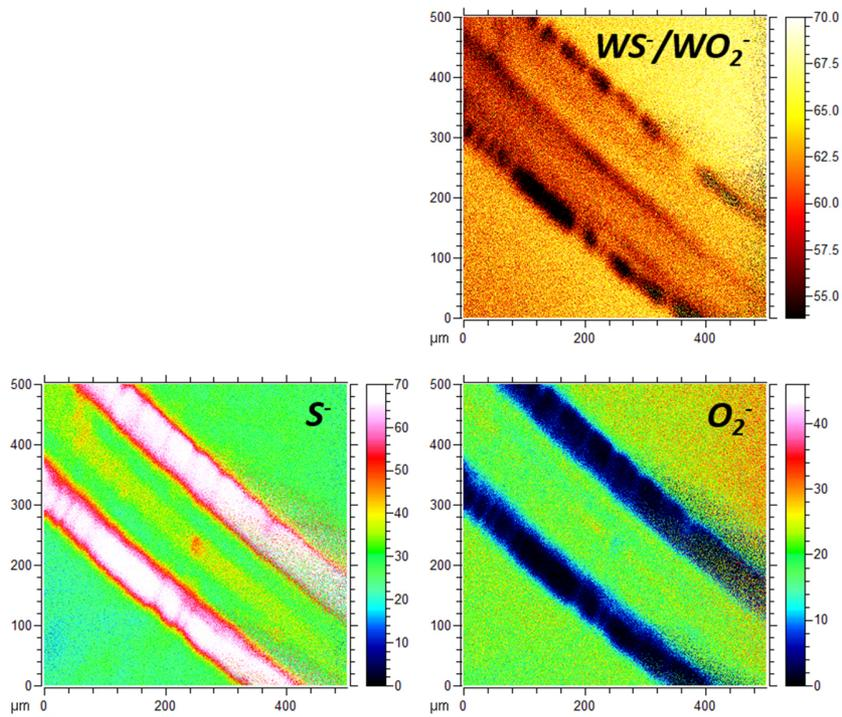
Figure 15: SIMS measurements of the wear track show clear evidence of the accumulation of a sulfide-based oxygen-depleted debris. It also highlights the in-situ formation zone in the middle of the wear track.
