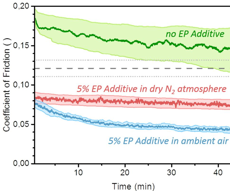
Figure 5: A  $\text{Si}_3\text{N}_4$ -ball vs. a Mo flat demonstrates a clear drop in friction in presence of the S-containing additive. Tests in dry  $\text{N}_2$ -atmosphere highlight the importance of the presence of oxygen in the contact.
