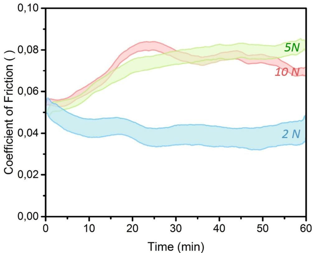
Figure 12: The in-situ formation also occurs on tungsten nitride coatings although the load bearing capability is limited.
