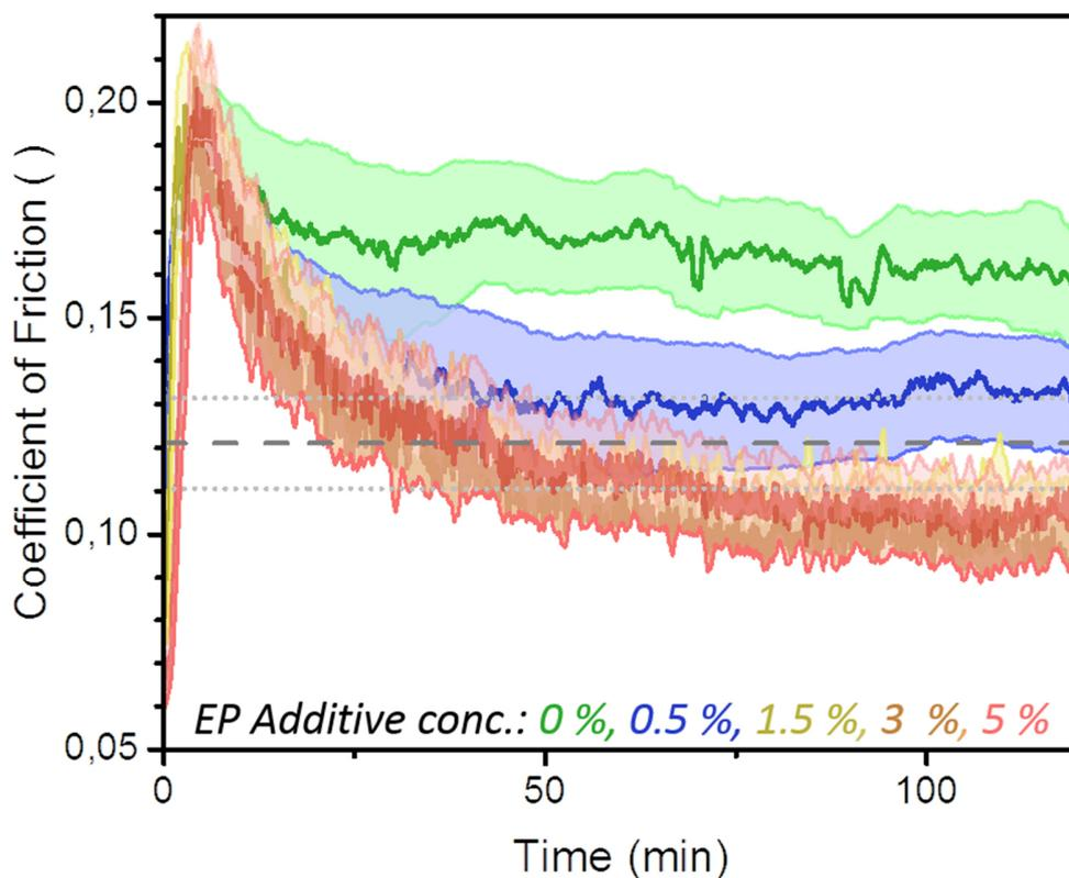
Figure 7: The coefficient of friction on metallic W is reduced by adding a EP-additive, but does not display the low friction we would expect of a  $WS_2$  lubricated contact.
