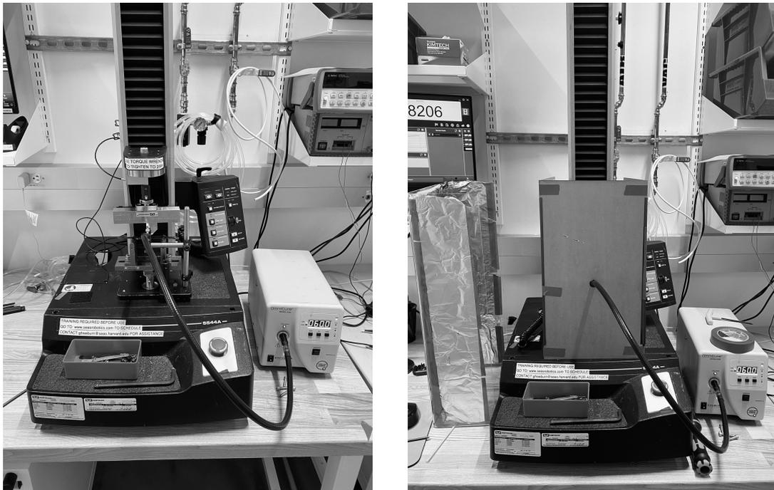
Figure 4.4.: Three-point beam test setup - front view (left) & enclosed view (right).
