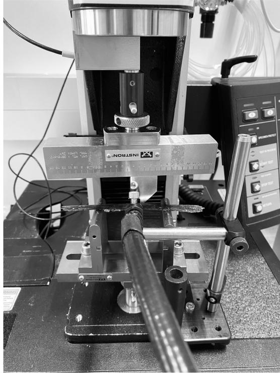
Figure 4.5.: Three-point beam test setup - beam and supports.
