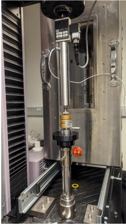
Figure 25: B3B-Testing setup for dynamic loading with the piezoelectric actuator.
