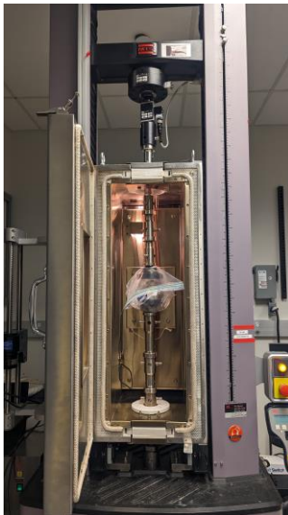
Figure 17: B3B testing setup for testing at elevated temperature and elevated humidity.
