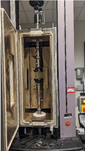
Figure 23: Test setup for elevated temperature
