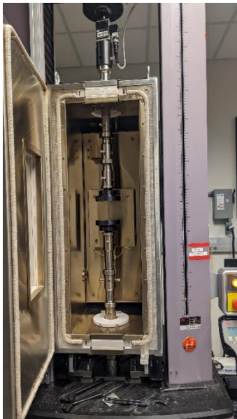
Figure 15: B3B testing setup including the temperature chamber for testing at elevated temperature.
