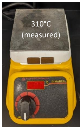
Figure 34: Image of the used hot plate for the local thermo-shock experiment
