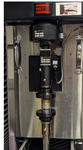
Figure 2: Picture of the used ball on three balls setup.
