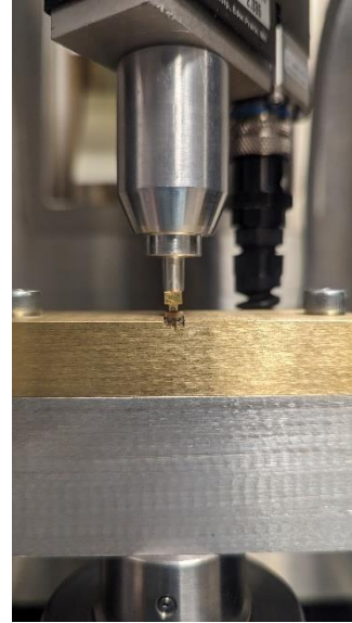
Figure 4: Picture of the used 3-point-bending setup.
