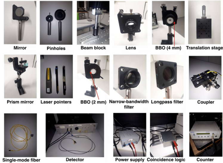
Figure 15: Required elements for the CHSH Bell Inequality test. Source: Valeria Saggio, "Experimental Violation of Bell Inequality"
