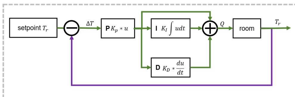
Figure 27: Functional diagram of a PID-controller (modified according to(Heinrich et al. 2020, p.163))
