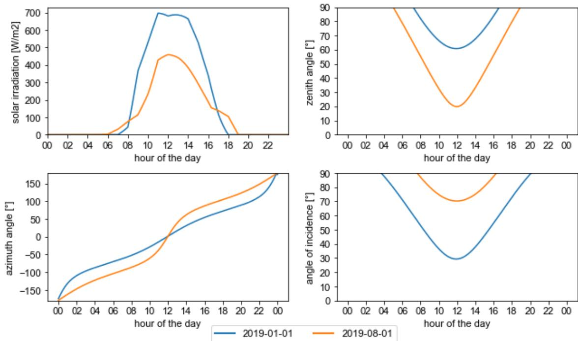
Figure 37: Solar angles and solar irradiation on tilted surface
