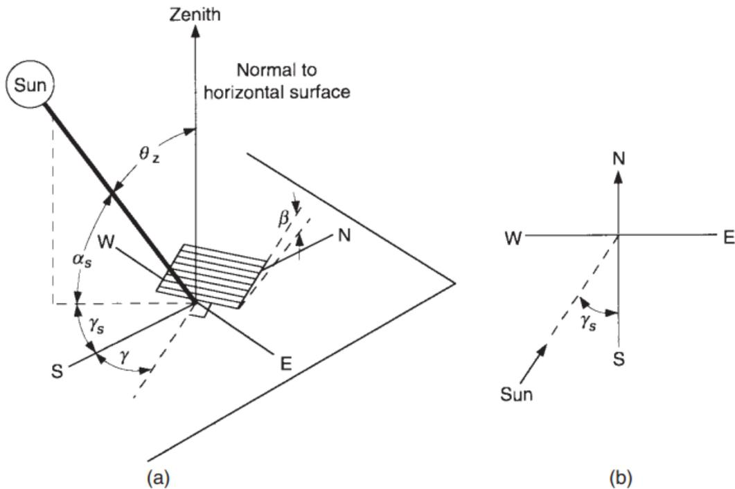
Figure 34: (a) Zenith angle, slope, surface azimuth angle and solar azimuth angle for a tilted surface. (b) Plan view showing solar azimuth angle (Duffie and Beckman 2013, p.13)
