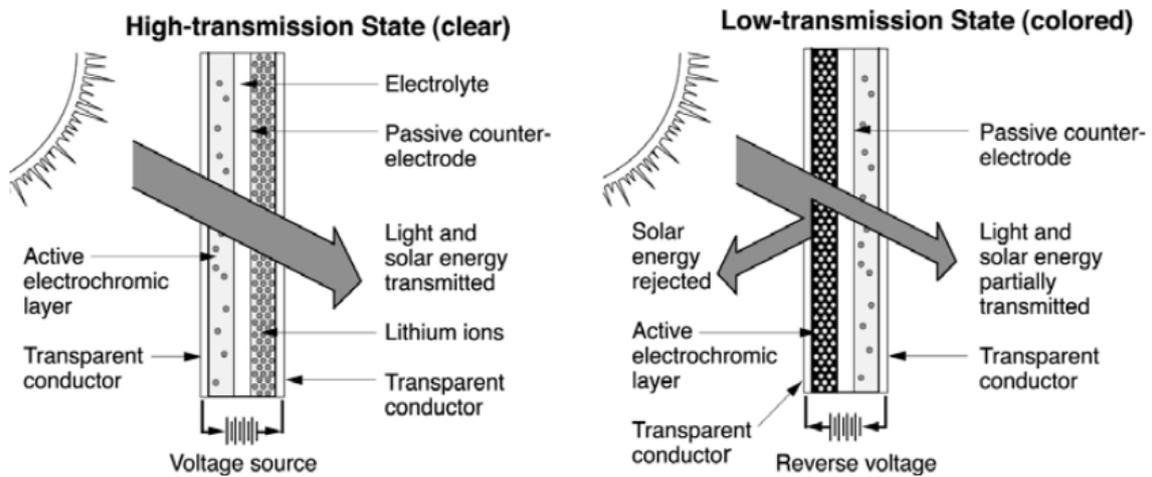
Figure 31: Diagram of a typical tungsten-oxide electrochromic coating (Lee et al. 2006, p.6)
