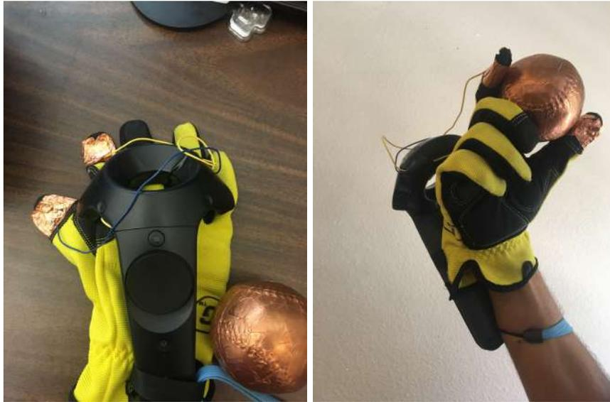
Figure 3.7: Left picture shows the empty glove controller that was used during testing. Right picture shows an example how the baseball is held and therefore sending a signal to the simulation.
