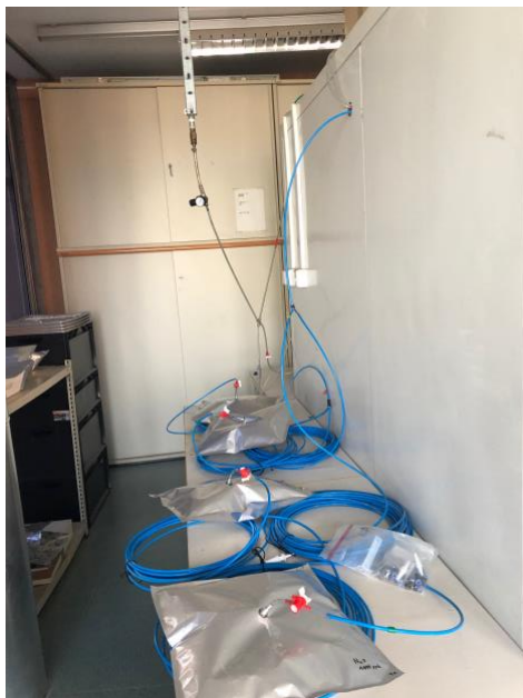
Branched inlet with gas bag set up outside of the temperature controlled room
