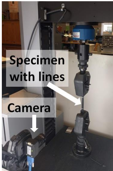
Figure 1: Experimental setup for the tensile testing. A high-resolution, monochrome camera was placed in front of the load frame to record images during each measurement. The strain was evaluated from the recorded images and it was further correlated with the force signal in order to obtain the stress-strain curve.
