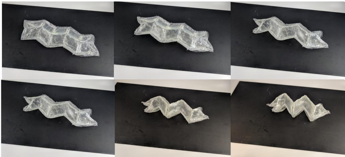
Figure 21. Examples of first prototypes of foldable membrane for origami organ on chip. Membrane used is PET as the material is quite resistant to temperature and easy to fill with gels and resins in order to observe mechanical folding.
