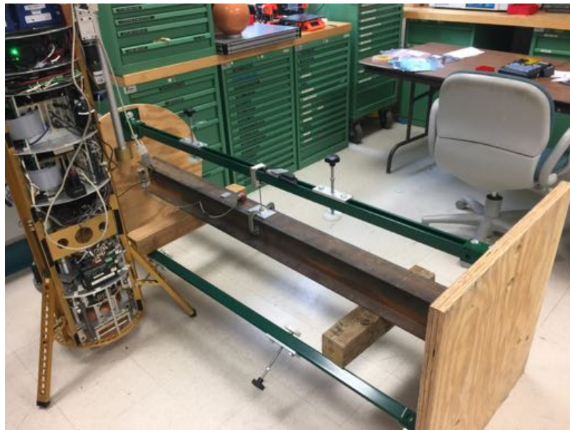
Figure 2: I-Beam mounted to the inertia measurement frame at its center of gravity
