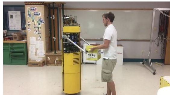
(b) The test person places the object on ballbot's raised arms (Time: 0:17)
