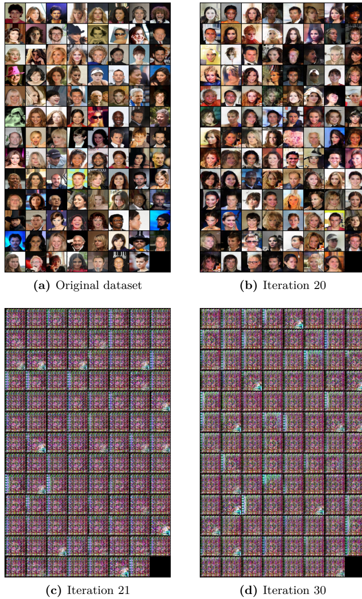
Figure 4.9: Generated output of a collapsed, single-instance GAN trained with the Lipizzaner gradient-based trainer: while the system works fine until iteration 20, it collapses in the following iteration and is unable to recover during the remaining training process.
