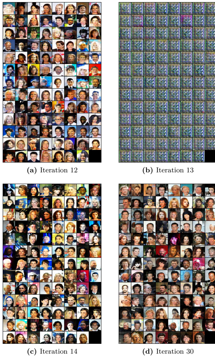
Figure 4.10: In contrast to the single-node results shown in Figure 4.9, a 2x2 gradient-based Lipizzaner grid is enough to overcome the otherwise critical system collapse observable in (c), and maintains a stable state until the end of the training process.
