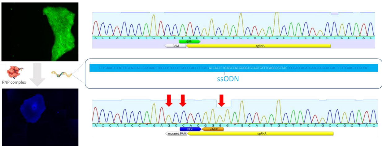
Figure 24 GFP to BFP conversion. A cell expressing GFP can be targeted via genome editing to turn into a BFP-expressing cell. Only one bp change is enough to convert GFP into BFP. Except for this essential 1 bp change, the introduction of two further silent mutations prevents re-cutting by the Cas9 enzyme and increases the fluorescence intensity (red arrows indicate the introduced modifications after HDR using the designed ssODN).
