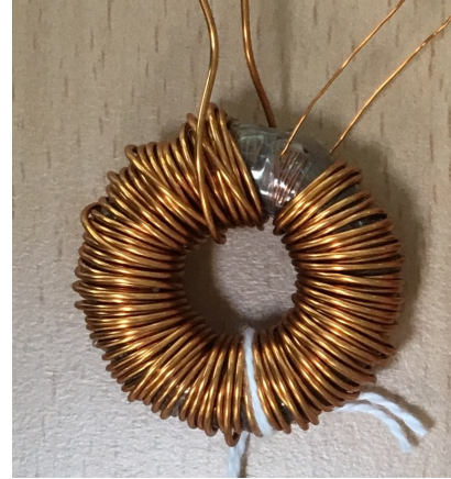
Fig. 5. Binder Jet Printed Ring Specimen with distributed windings.
