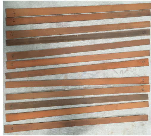
Fig. 3. BJP Specimen # 5 Mechanically Cut into Strips.
