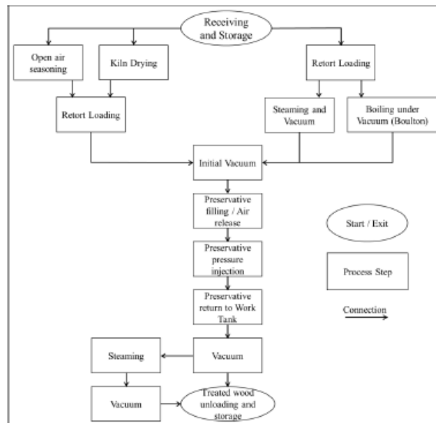
Figure 1. Example Process Flow Chart: Full-cell and modified full-cell pressure treating process for treated lumber [5].
