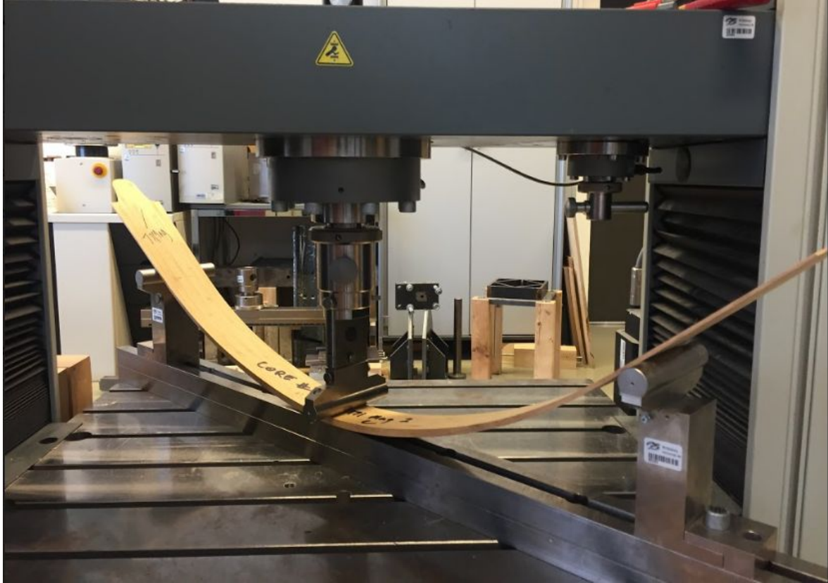
Figure 13: Max bending test on bamboo ski cores
