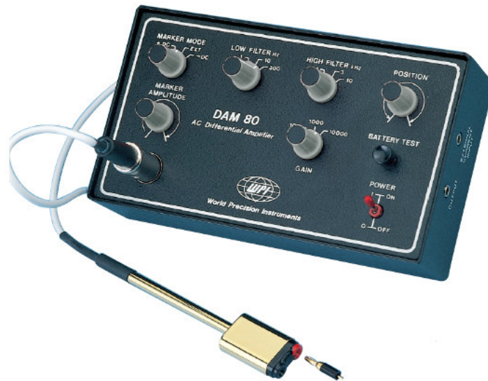
Figure 3.2: Graphic of the DAM80. The low pass filter can be set between 0.1 Hz, 1 Hz, 10 Hz and 300 Hz and the high pass filter between 0.1 kHz, 1 kHz, 3 kHz and 10 kHz. Moreover, the amplification factor can be chosen between 100, 1000 and 10 000. Further features are not used in this thesis [60].
