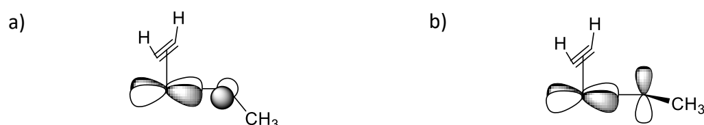
Figure 17: Orbital interaction between a) W and S at dh(methyl thiolate) = 0.0° and b) W and S at dh(methyl thiolate) = 90.0°.
