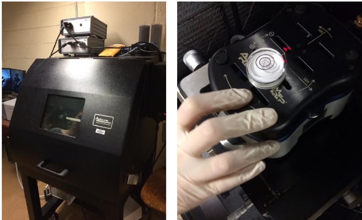
Figure 29: External view of the installed AFM instrument utilized in the study (left), and the head being adjusted for the height (right)
