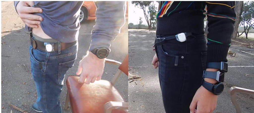
Figure 34: Different positions of sensors on different participants. The sensor is visibly lower on the hip on the left participant than on the right.
