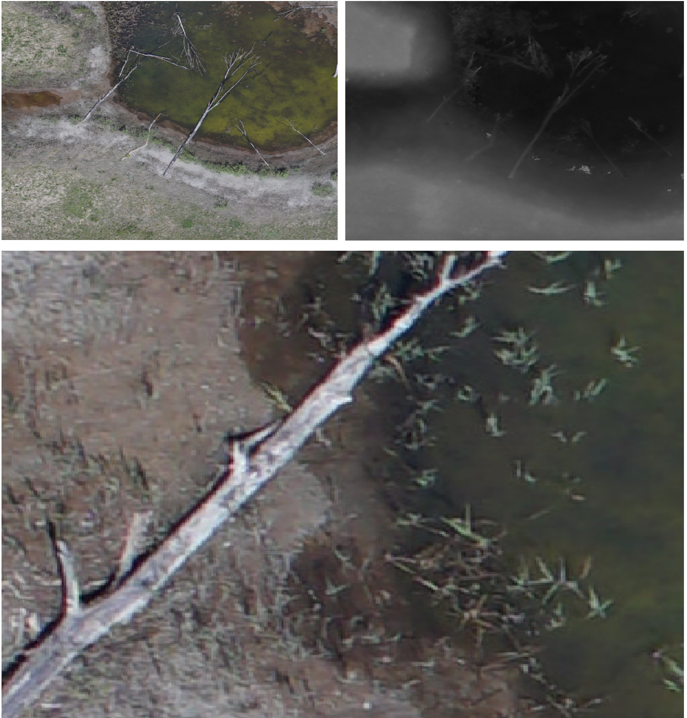
Figure 13: Examples of the orthoimage and DEM created during the repeated processing of the Bramor ppK sUAS in Carinthia, Austria. Top left is a subset of the orthophoto, top right is the DEM, and bottom is a zoomed in view of a portion of the orthophoto in the top left.
