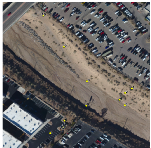
Figure 8: GCP Locations used in correction and accuracy evaluation.
