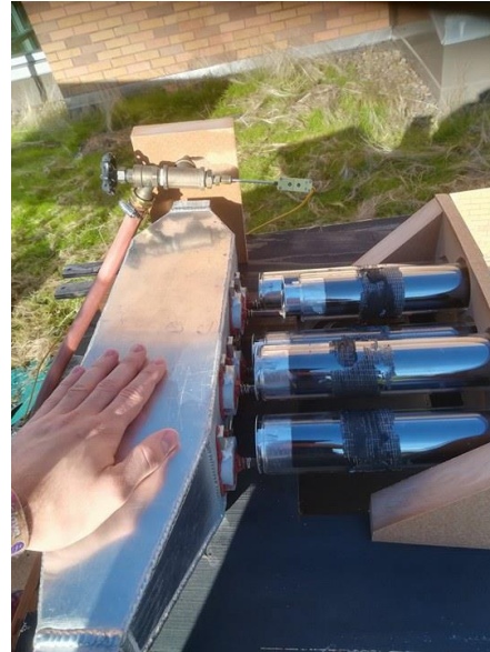
Figure 17. Heat exchanger evacuated tubes.
