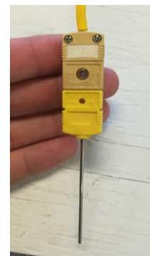
Figure 10. Type K thermocouple used for ambient temperature measurement
