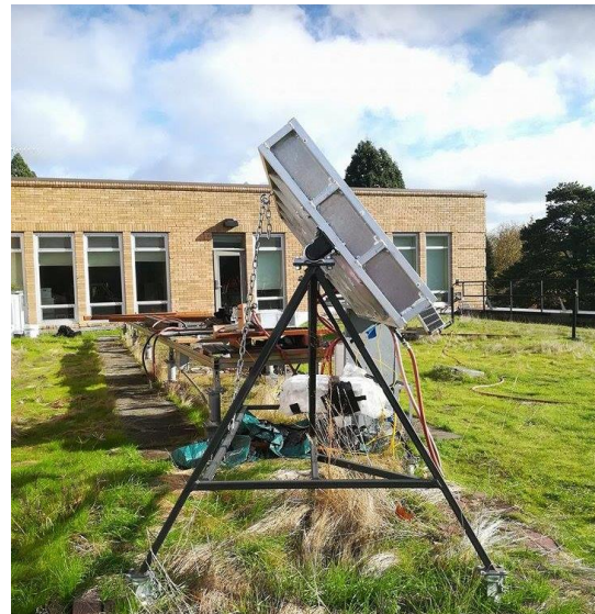
Figure 19. Flat plate solar collector with adjusted angle for November conditions.
