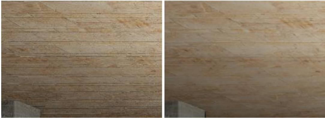
Figure 27: Comparison of compute vs fragment shader rendering. Left image: compute shader. Right image: fragment shader. The missing anisotropic filtering is clearly visible.
