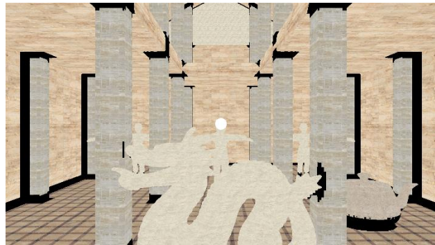
Figure 22: Visualization of the world id field. All black regions are „uncertain“, i.e. intersections between different field influences.
