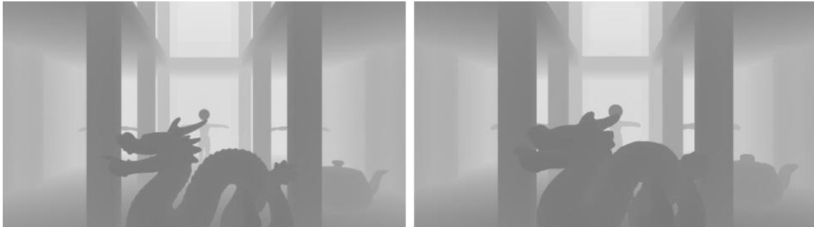
Figure 21 : The depth buffer after sphere tracing. On the left, the full algorithm with all optimizations is run. On the right only the world distance field is polled. The conservative distance estimate is clearly visible by the bulkiness of the dragon in the front. Due to the low resolution of the field, details like the dragon's scales disappear.
