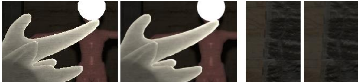
Figure 28: Comparison of a rendered image with and without TAA. The left image pair demonstrates TAA's blurring and anti-aliasing effect. The right image pair shows shadow bleeding artefacts from undersampling. These artefacts are visibly reduced through temporal anti-aliasing.
