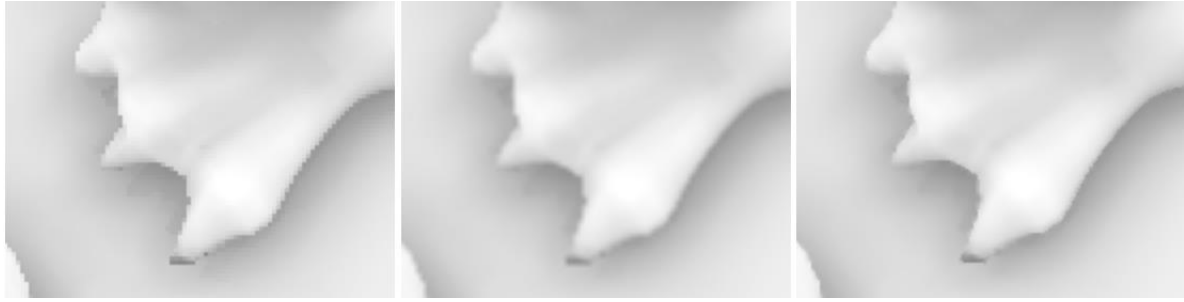
Figure 26: Comparison of different upsampling techniques. The left image is bilinear upsampling, the pixelization issues are clearly visible at object edges. The center image was upscaled with a Gaussian blur using a 3x3 kernel. The pixelization disappears, but the AO factor of different objects gets smeared across object boundaries. The right image is upscaled using bilateral filtering. The pixelization issues disappear, but the object boundaries stay sharp.
