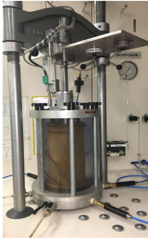
Figure 23: Assembly of Triaxial Cell with Respective Pipes
