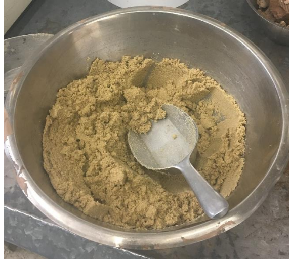
Figure 10: Fine Sand mixed with given water content ( w = 15\% of the initial mass).
