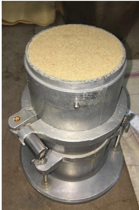
Figure 15: Wet Sand Inside proctor device with height of 20.2 cm
