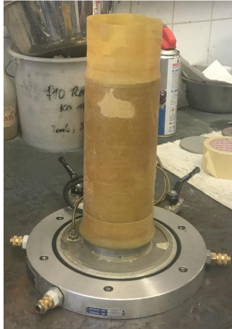
Figure 19: Rubber Membrane(s) Covering the Sand Cylindrical Specimen
