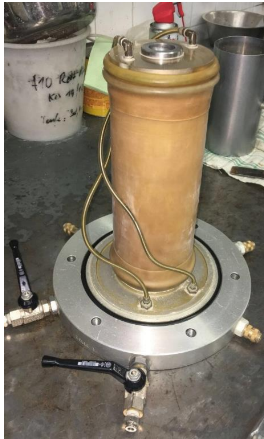
Figure 20: Placement of Filter Bases with Pipes
