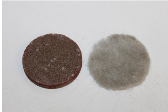
Figure 14: Thin Filter stone and Filter Fleece (diameter = 10 cm)
