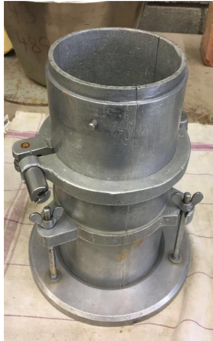
Figure 11: Proctor Compaction Apparatus
