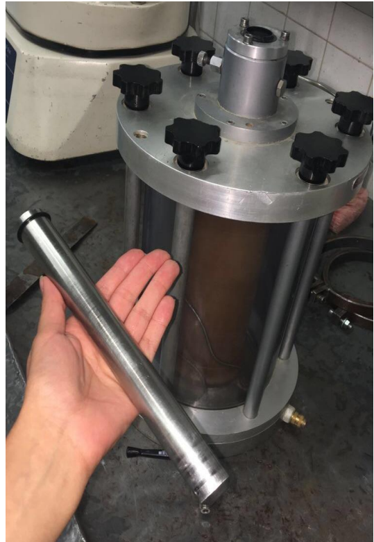
Figures 21 and 22: Placement of Loading Frame Cover and Loading Ram
