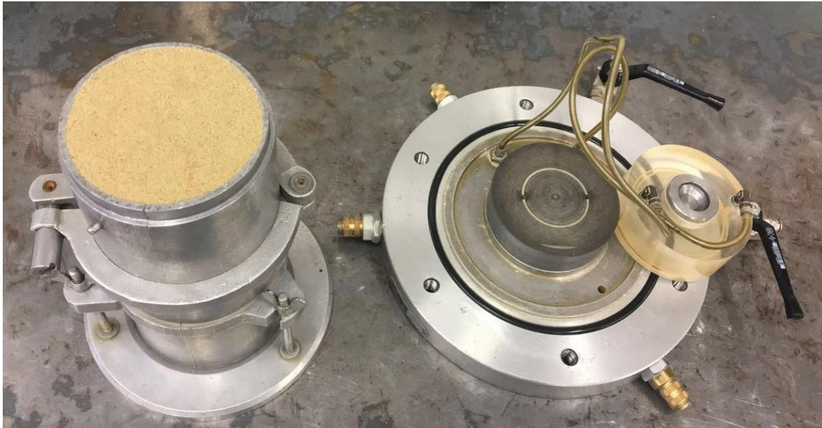
Figure 16: Proctor device with sand and loading frame base
