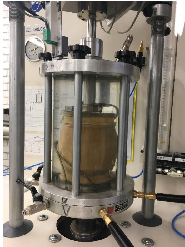
Figure 24: Probe Bulging at Loading
