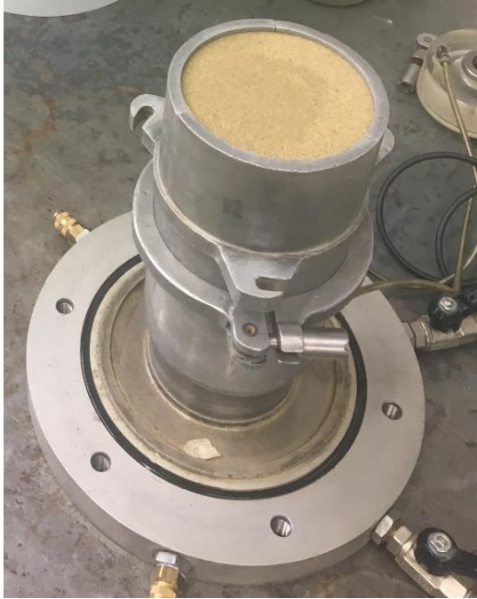
Figures 17 and 18: Placement of Cylindrical Sand Sample
