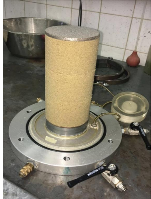
Figures 17 and 18: Placement of Cylindrical Sand Sample
