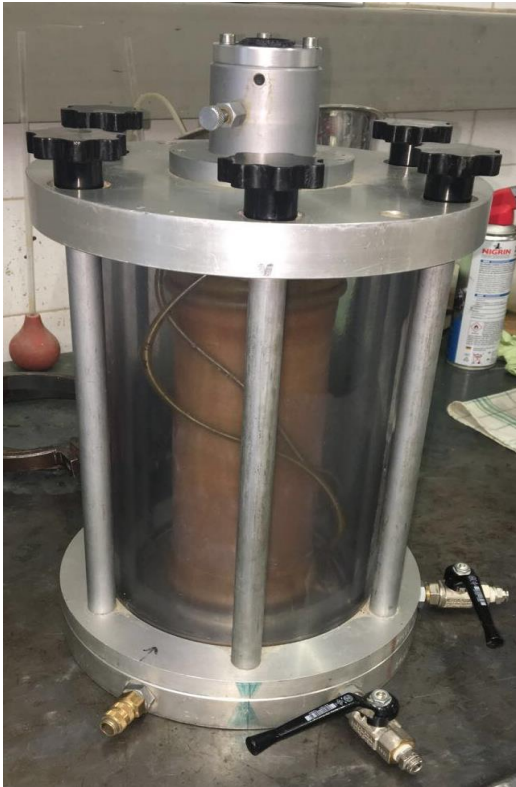
Figures 21 and 22: Placement of Loading Frame Cover and Loading Ram
