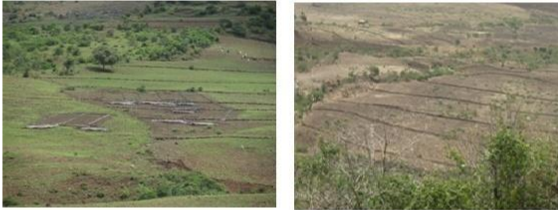
Figure 2 Erosion plot experiments (left) and SWC structures (right) at the treated watershed
