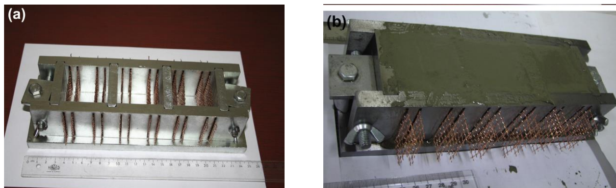
Figure 19: Copper mesh pre-arranged in a customized mold (Teomete, 2014)
