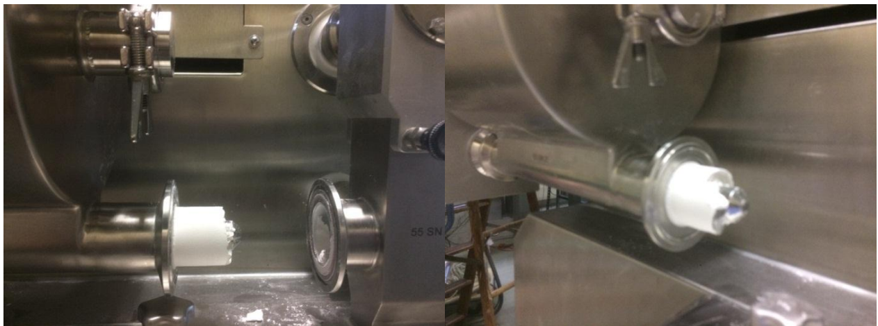
Figure 20: Avicel PH 105, stuck inside the feeding auger due to its cohesive powder properties, necessitated manual cleaning
