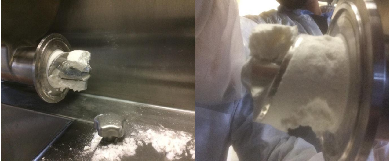
Figure 21: Solka Floc, stuck inside the feeding auger due to its cohesive powder properties, necessitated manual cleaning
