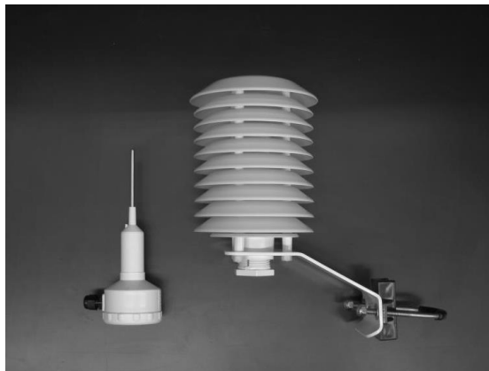
Figure 28 RTD temperature probe and radiation shield for ambient temperature measurement (Boyd, 2015)
