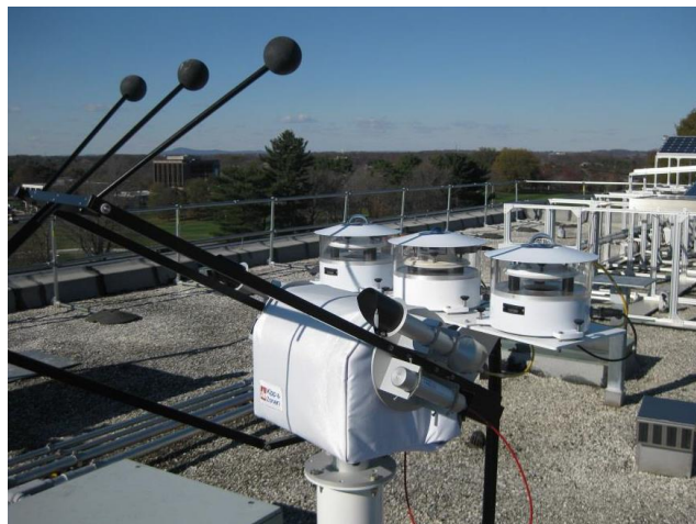
Figure 31 Pyrheliometers mounted on the side of the solar tracker also showing the diffuse measuring pyranometers (left and right) and the IR measuring pyrgeometer (center) (Boyd, 2015)
