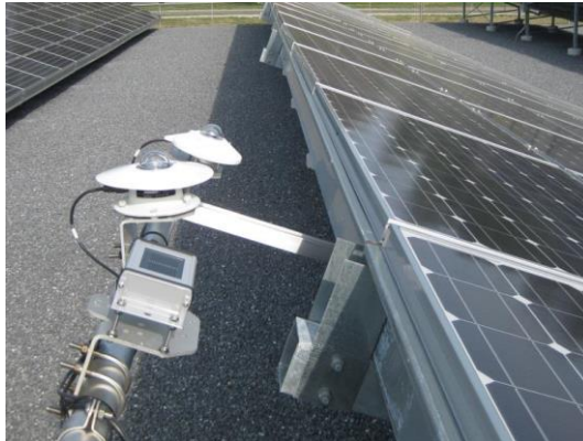
Figure 27 Irradiance sensors at the ground array measuring G_{poa} and GHI (Boyd, 2015)
