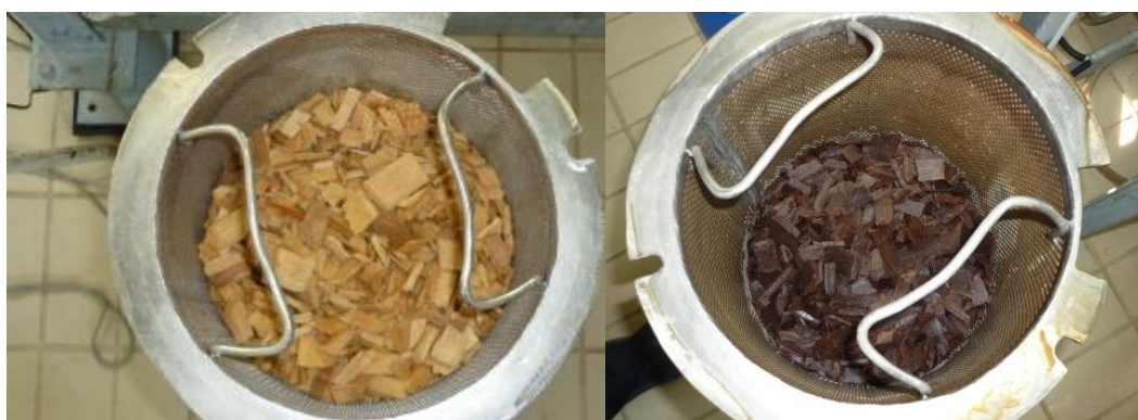
Figure 1: Wood chips before (left) and after organosolv treatment (right)
