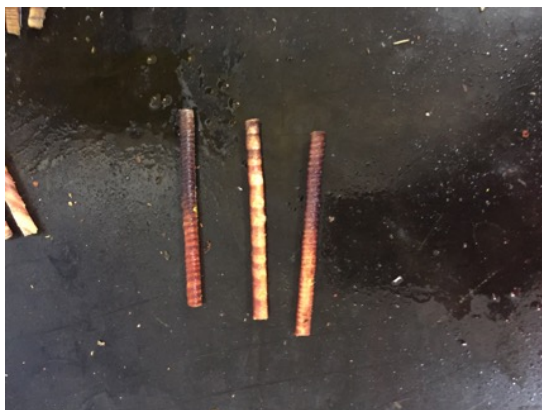
Figure 7: Samples with applied heartwood indicator
