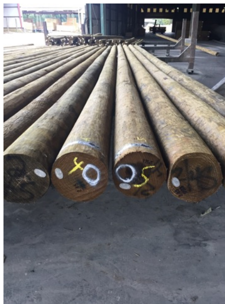
Figure 4: Poles on drip pad
