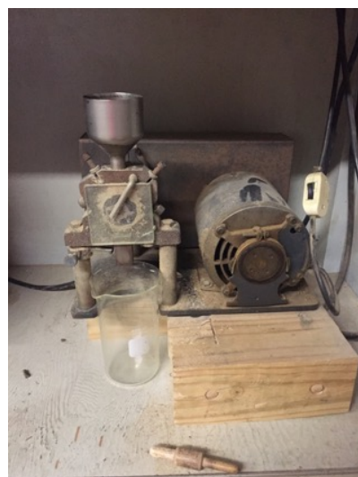
Figure 10: Grinding of the core samples with a grinder
