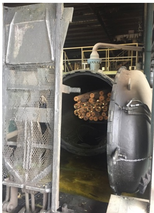
Figure 2: Loaded treatment cylinder
