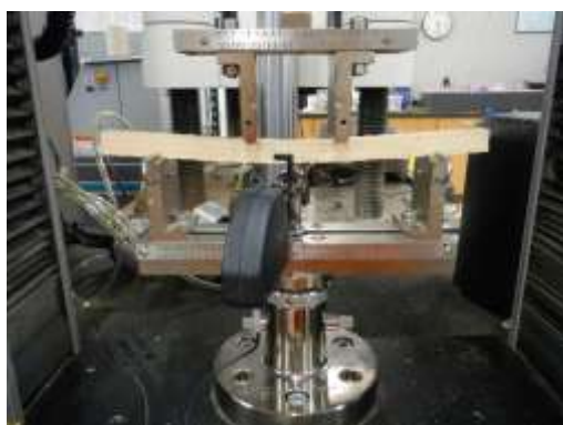
Figure 27: testing machine with 4-point bending apparatus and sample
