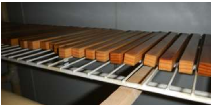
Figure 19: seasoning of all samples in the seasoning chamber (25°C, 65% RH)
