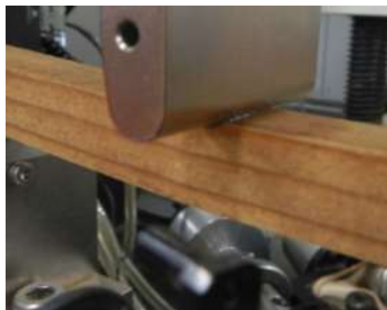
Figure 51: Diesel comes out of the beam during the testing
