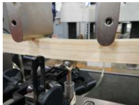
Figure 29: loading pins that apply force on the beam, additional measuring device under the beam
