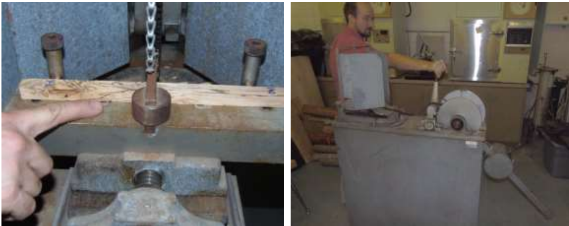
Figure 6: Pendulum toughness testing, showing sample ready for testing (left) and lever that is pulled to release pendulum (right). Toughness is calculated as a function of distance travelled by the pendulum after breaking the sample (Forest Products Laboratory, 1961)
