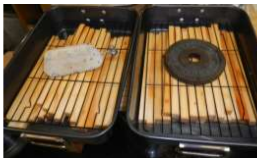
Figure 16: mesh and weight put on top of the samples in the pans as preparation for the Boultonizing process
