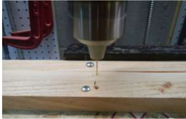
Figure 9: drilling the 1mm holes for the half of the samples
