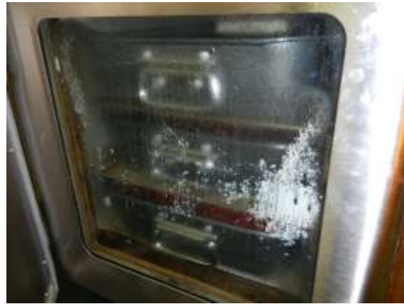
Figure 18: during the process, condensed water on the glass door, three pans with two layers of samples
