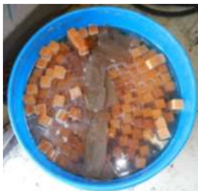
Figure 15: rewetting of the samples, no or only slightly floating at the end
