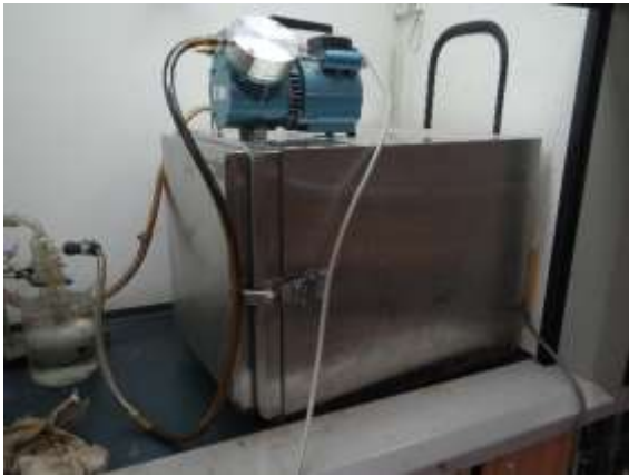
Figure 17: vacuum oven for the Boultonizing process
