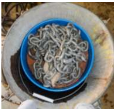
Figure 13: ballast put on the samples in the bucket for a complete submerge
