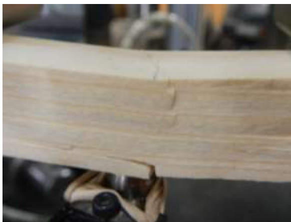
Figure 50: tension and compression failure during 4-point bending
