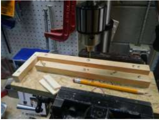
Figure 8: jig for drilling the holes for the through-boring attempt
