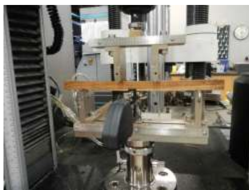
Figure 27: testing machine with 4-point bending apparatus and sample
