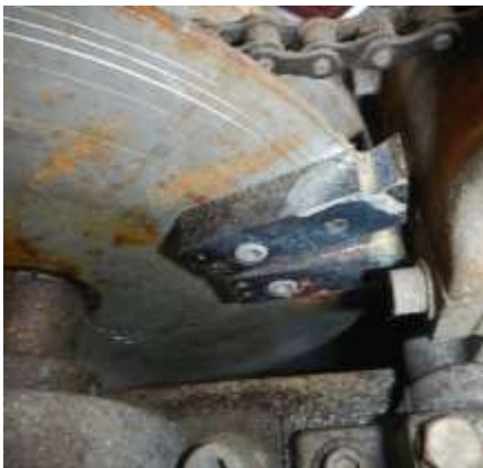
Figure 22: adjustment for the prepared samples of the testing machine for toughness (company: Wiedemann, Baldwin); the picture shows the upper part of the pendulum
