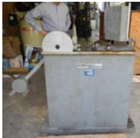
Figure 23: adjustments for the prepared samples of the testing machine for toughness testing (company: Wiedemann, Baldwin); the deflection of the pendulum can be seen and the hand lever
