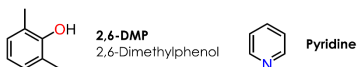
Figure 4. Chemical formulas of the monomers used in the iCVD and oCVD depositions of this study. The structures are labeled by their respective abbreviations (given in bold, capital letters), with their common names being stated below.
