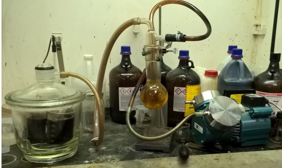
Image 5: Apparatus used for vacuum impregnation, pic.: Stelzer R.
