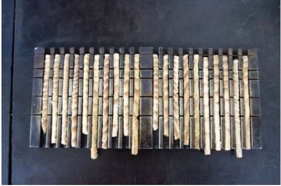
Image 15: 20 Core samples taken from treated lumber
