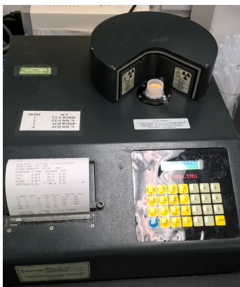
Image 24: Asoma Ametek 200 XRF – Analyzer, pic.: Stelzer R.
