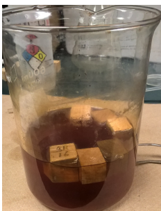
Image 4: Preparation of gum test – blocks in 2,47% solution of recovered creosote, pic.: Stelzer R.
