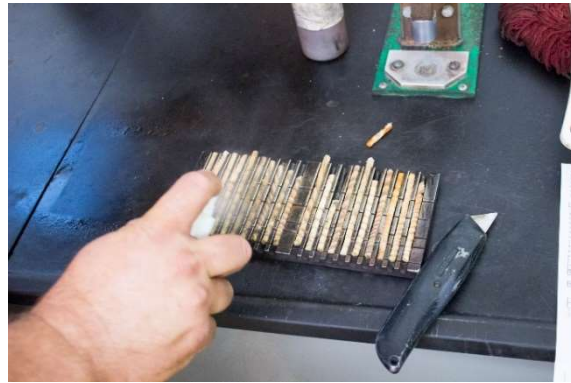
Image 17: Apply indicator spray for copper on core samples
