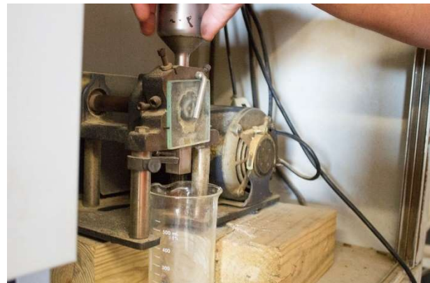
Image 19: Grinding dried cores for XRF – measurement
