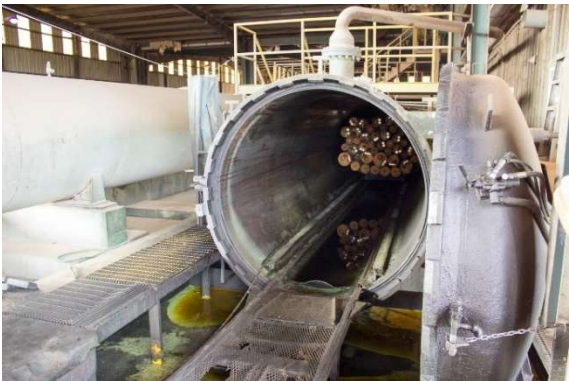
Image 10: Treated lumber pressure cylinder
