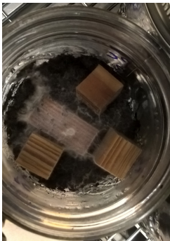
Image 7: Little growth of fungi after a week of application of pine test-blocks, pic.: Stelzer R.
