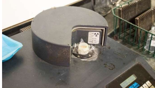
Image 21: Sample ready for XRF – measurement
