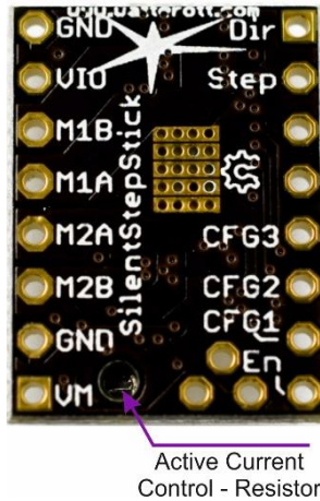
Figure 4-11: Trinamic TMC2100 – Stepper Motor Driver – Active Current Control
